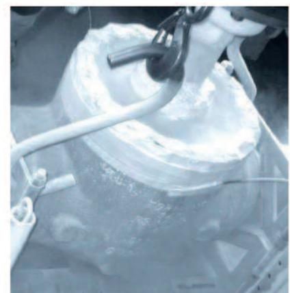
LTG3 - control valve under cryogenic test
