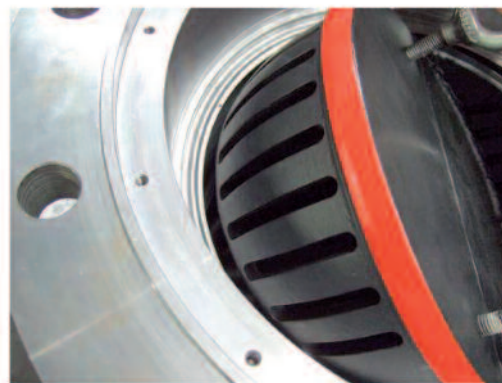
Anti-cavitation disc design
