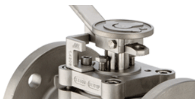
AZ plug valves are fitted with cast, rust proof position indicators The position indicator is securely welded to the plug to prevent it from working loose.
