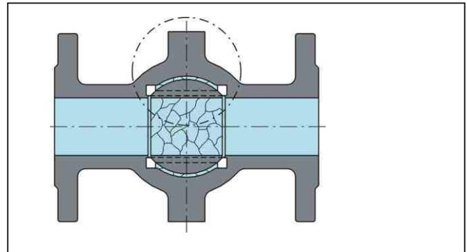
**Solid matters can damage the sealing rings.**
