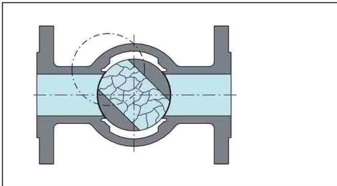
**By crystallizing and sedimentary products:** Even by coagulation **no danger for sealing or operation of the plug.** There are **no dead spaces, therefore products cannot accumulate or stay behind.**
