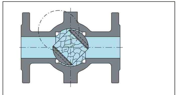
**By crystallizing and sedimentary products:** **Danger of coagulation because of dead spaces, therefore difficult operation of the ball.** Danger of damaging the sealing rings. **Torque increase** through one-sided pressure.
