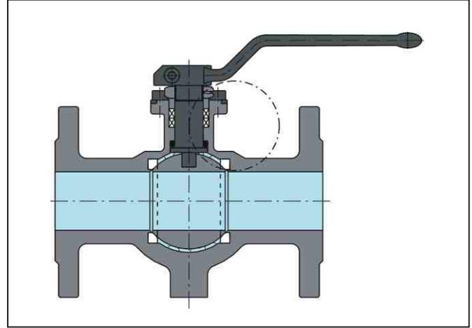
**Sealing surface of the ball in open position fully exposed to aggressive products (because of dead spaces).**
