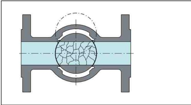
**The plug is totally encircled and protected by the PTFE sleeve. Solid matters cannot damage the sleeve, because this sleeve is non-adhesive.**
