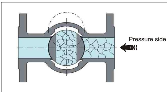
**Ball Valve with PTFE sealing ring**
